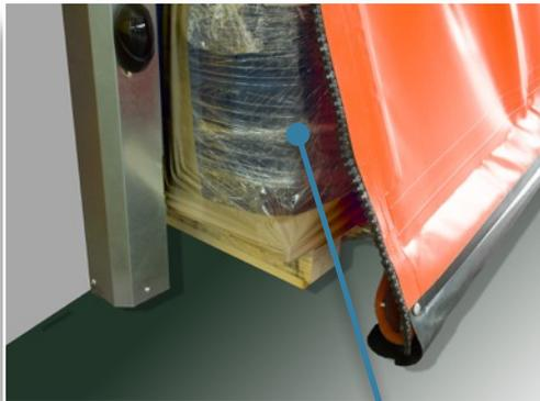
*THE SELF-REPAIRING SYSTEM ABSORBS ENERGY ON IMPACT TO THE CURTAIN, ALLOWING IT TO TEAR AWAY FROM GUIDES AND AVOIDING DAMAGES. AFTERWARDS THE CURTAIN IS RESET AUTOMATICALLY FOR THE FOLLOWING OPENING*
