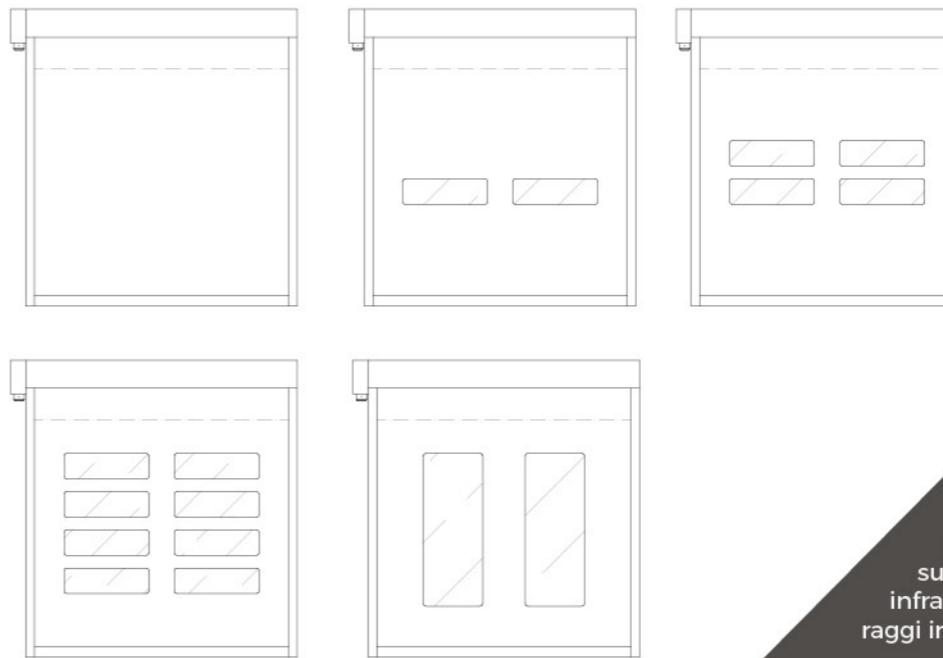
**Safety:** safety edge of electro-conductive rubber sensitive to pressure on the bottom of the curtain and single beam infrared photocells or light curtain with crossed beams.
